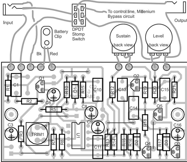
*D&R Comp - Parts Placement for Ross Compressor (tm) clone - wiring is identical!*
