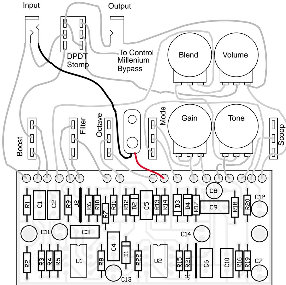
Board is sized to fit inside a Hammond 1590BB, but with five toggle switches and four controls, it's going to be a very tight fit. I recommend the Hammond 1590DD, which has a much larger face, suitable for more controls.
