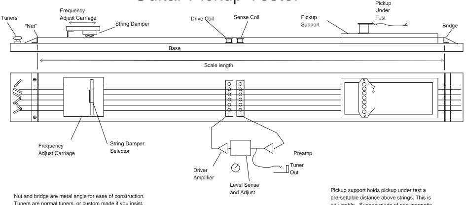
Tuners are normal tuners, or custom made if you insist. Frequency Adjust Carriage lets you adjust string frequency by moving a sliding "fret" (another angle) up and down strings. Also lets you adjust which string is NOT damped by the damper mechanism. There are many ways to do this.
