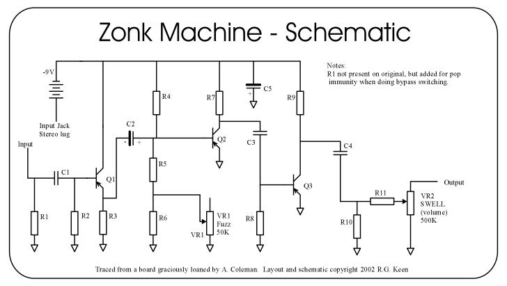
This has a couple of consequences. First, even modest signals at the base will turn Q3 off entirely, making for hard clipping. Second, like the Dallas Rangemaster, the characteristic curves for germanium near cutoff are distinctly nonlinear, providing some soft distortion. All from changing the value of the bias resistor.
