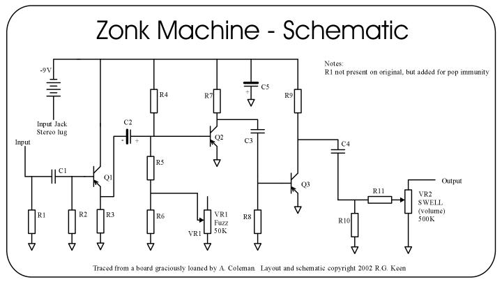
This is the schematic of the whole circuit, less the input/output jacks and bypass switching arrangements, which have been left out for clarity about the circuitry. The jacks, controls, and bypass switching are all shown in the wiring diagrams that follow.
