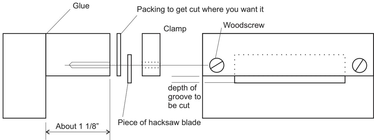
Special purpose tool for cutting gold piping groove in finished cabinet.
