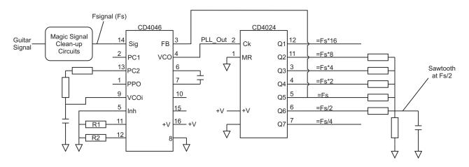
The fun starts with a Phase Locked Loop, a CMOS chip (CD4046) that can make its internal square wave oscillator follow a square wave input at the same frequency, and track it around as the input signal's frequency rises and falls.
