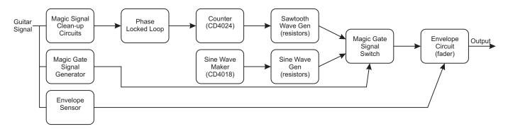
The envelope sensor makes a signal that is proportional to your guitar's loudness, and then sends it to the envelope circuit, which is an electronic volume control or fader. When the envelope is high, the volume control is high, when the envelope is low, the output volume is low. You may be wondering why if we have an envelope follower we need a gate. It's because gates are on/off, not messing about almost on or off. You want the space between notes to be completely silent.
