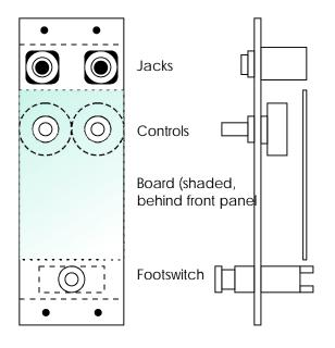
Note that the jacks are a big space eater. It might make sense to make the on-effect jacks be 1/8" phone jacks and interconnect between effects with 1/8" phone plugs and RG174 cable, then put a 1/4" jack out on the end panels to take the guitar cord and the cord to the amp.
