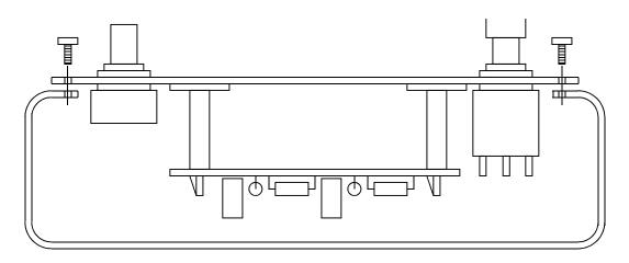
The effects mount inside like this. The boards are mounted on adhesive standoffs. The controls and switches, including footswitch, mount in holes drilled in the aluminum plate. If you're careful, you can stand the board off the aluminum enough to put small pots between the board and the aluminum front panel and get LOTS of controls in there.
